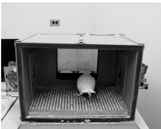
Figure 3. The front view of the apparatus used to present the object stimuli in Experiments 1–3. Both humans and pigeons saw the same stimulus tableaux; the door to the box was closed for the pigeon subjects and remained open for the human participants. From “An Automated Apparatus for Presenting Depth-Rotated Three-Dimensional Objects for Use in Human and Animal Object Recognition Research,” by A. Friedman, M. L. Spetch, and I. Lank, Behavioral Research Methods, Instruments, & Computers , 35, p. 345. Reprinted with permission.
